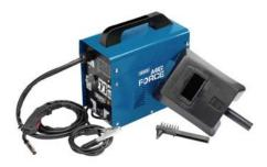
Uses flux cored wire. During the weld process the flux melts and protects the weld, therefore no gas is required to shield the weld pool. Ideal welder for use outdoors in windy conditions. Features: Non - live direct fit safety torch, Variable wire speed control, Thermal overload protection, Earth clamp, Supplied with spool of flux cored wire, chipping hammer/brush and face mask.
