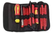
Expert quality, tested to 10kV, suitable for working on live circuits of 1kV AC and 1 5kV DC SCVM steel blades hardened, tempered and chemically blackened. Interchangeable insulated blades deep set into handles precision or high torque types - for total safety. Mains tester included in set. Supplied in storage roll. Display packed.
