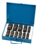
Draper Expert HI-TORQ® 6-point 1/2" square drive deep sockets. Overall length 78mm Forged from chrome vanadium steel correctly hardened and tempered, with a black phosphate finish for corrosion protection. Hole for receiving ball retainer. Supplied inside a steel x Sockets: 15, 16, 17, 18, 19, 21, 22, 24, 27, 30, 32mm
