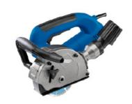
Features: Expert Quality, Adjustable cutting width 8 - 28mm, Adjustable cutting depth 10 - 30mm, Soft start, Dust extraction outlet, Supplied with 2 x diamond blades, side handle chisel and 3M cable with BS plug
