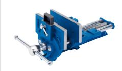
Robust, close grain cast iron woodworking bench vice fitted to allow jaw to slide freely along the buttress thread screw. When used with a bench stop, larger workpieces can be held using the adjustable front dog. Carton
