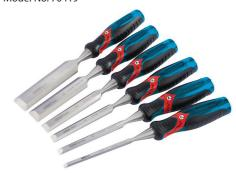
Expert Quality, full - length bevel edged blades manufactured from chrome vanadium steel hardened, tempered and finely ground. The solid impact - resistant soft grip handle allows the 'Pound Thru' striking end cap to be struck without causing damage. Supplied in an Content: 6 x chisels: 6, 12, 19, 25, 32, 38mm
