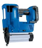
Features: Part of the D20 series. Single or contact firing, Safety contact tip, Supplied with 1x 2Ah battery and charger. D20 interchangeable battery system allows you to combine one battery with any of the tools within the D20 series. | Battery - D20 20V Li-ion | Firing Rate - 60 per min | Nail Gauge - 18 | Nail Length - 20-50 | Staples - Type 90 | Staple Length - 19-40 | Magazine Capacity - 100 | Batteries Per Item - 1 x 2Ah | Charger Type - 1.65A | Supplied in Case - Yes | Weight (bare
